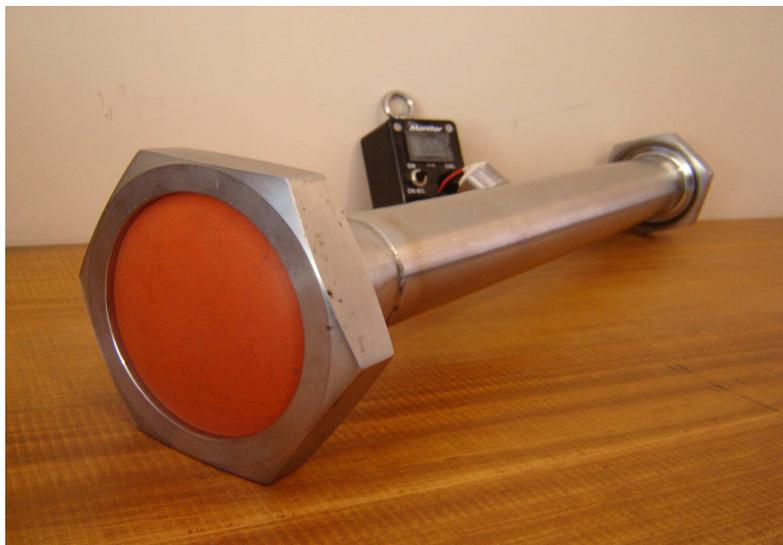
1000ml test cell with silicone Membrane in place
